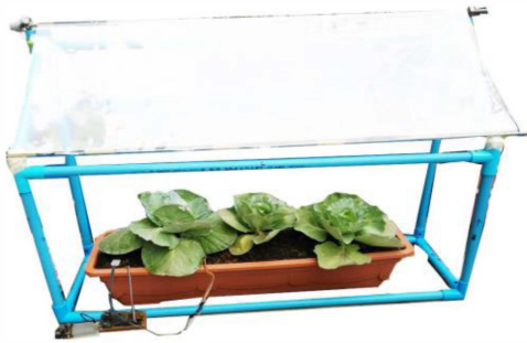
Fig. 5 A plant plot as a prototype installed with watering and roofing system and with sensors
