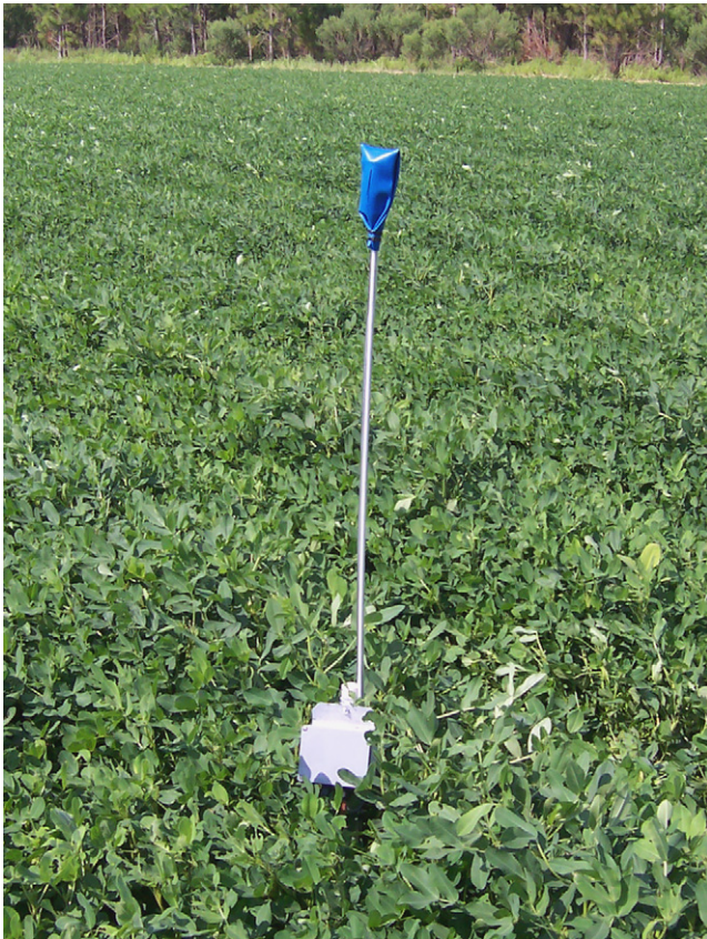
Fig. 2 – Modified smart sensor node with raised transmitter in a peanut field.
