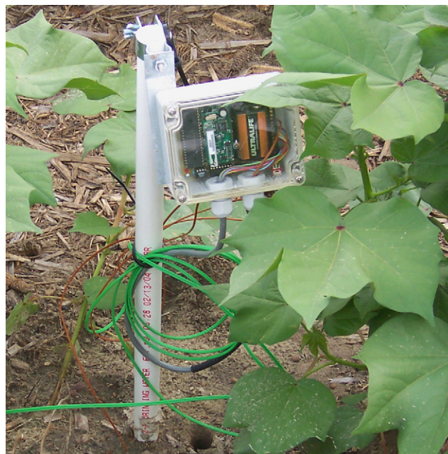
Fig. 1 – A smart sensor node which includes three soil Watermark ® sensors and two thermocouples installed in the NESPAL field a few weeks after planting of cotton.
