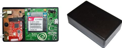
Figure 7: Final Access Point device.
