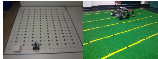
Fig. 12. Validation of the A* algorithm in Brazil, with NXT camera (left) and sensors included in Colombia (right).
