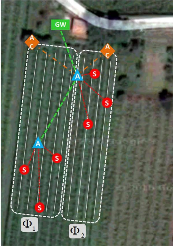
Fig. 6. Wireless architecture deployed in the test-field for experimental validation.
