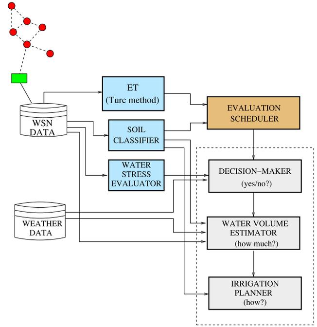
Fig. 2. Block-scheme of the proposed DSS.
