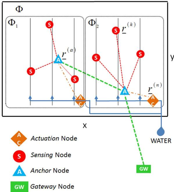
Fig. 1. WSAAN architecture based on a hybrid star-mesh topology.
