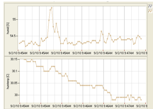
Figure 7. Output Graph Showing the temperature and humidity data of a node placed in a farm using MoteView Software.
